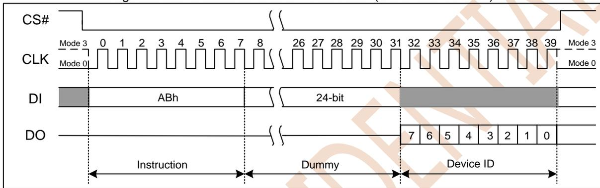
Figure 7.27a Release Power-down / Device ID(SPI Mode)
