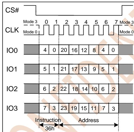
Figure 7.40b Individual Block/Sector Lock Instruction(QPI Mode)
