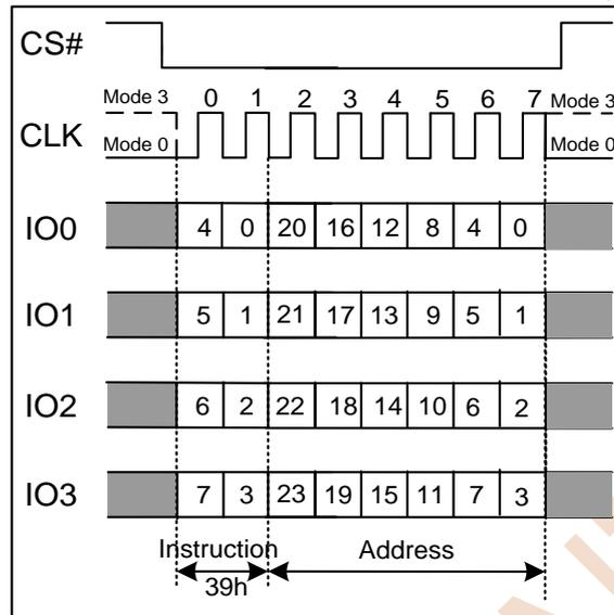
Figure 7.41b Individual Block/Sector Unlock Instruction(QPI Mode)
