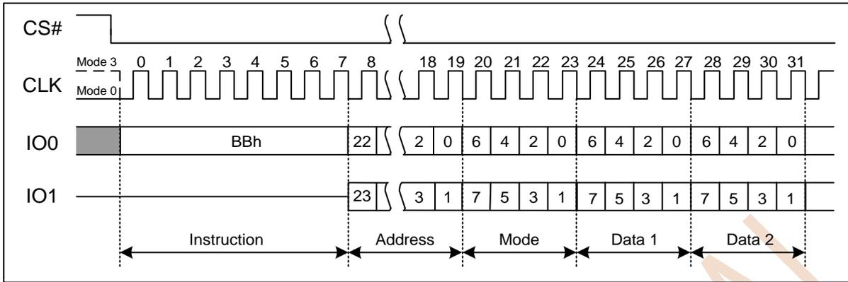
Figure 7.18a Fast Read Dual I/O Instruction (Initial command or previous M5-4≠10)
