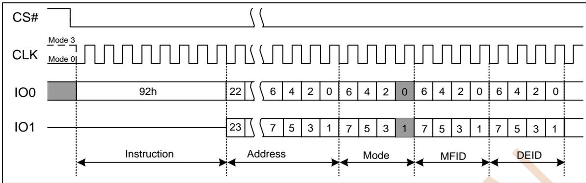
Figure 7.34 Read Manufacturer/Device ID Dual I/O Instruction
