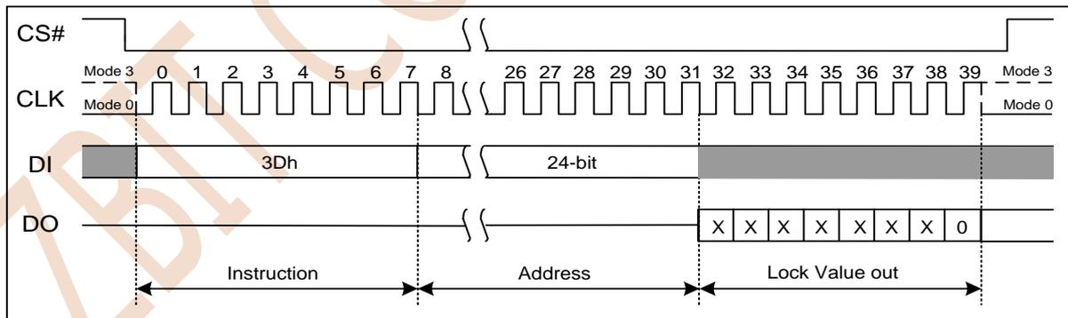
Figure 7.42a Read Block Lock Instruction(SPI Mode)
