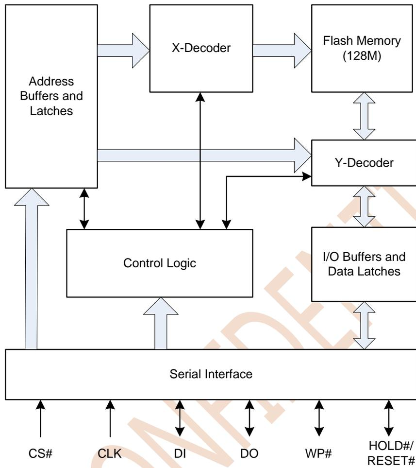
Figure 2.1 Block Diagram
