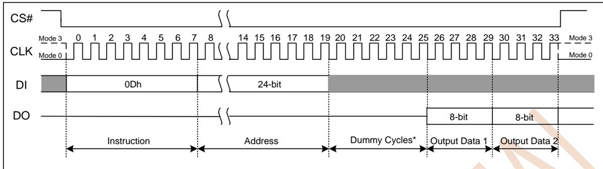
Figure 7.15a DTR Fast Read Instruction (SPI Mode)
