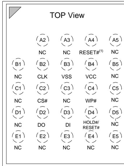
**Figure 3.4 24-BALL TFBGA (5x5 ball array)**
