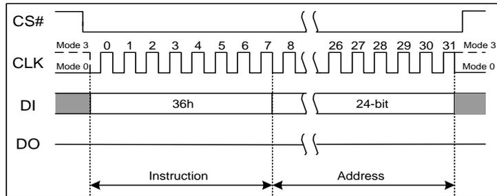
Figure 7.40a Individual Block/Sector Lock Instruction(SPI Mode)
