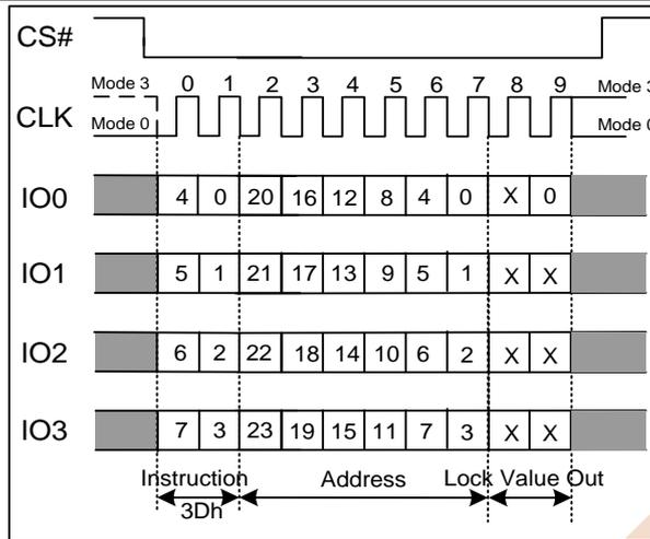
Figure 7.42b Read Block Lock Instruction(QPI Mode)
